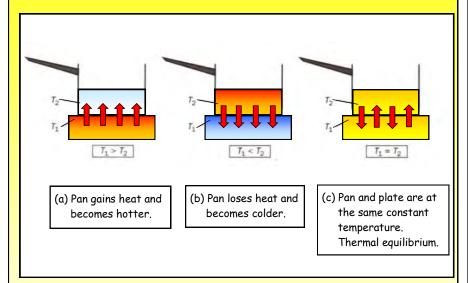
In (a) a pan containing water is placed on a very hot metal plate. Heat flows from the plate to the pan, which becomes hotter, so the temperature  $(T_1)$  of the plate must be greater than that of the pan  $(T_2)$ .
