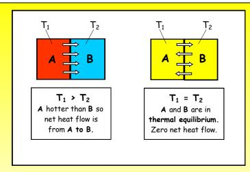
If two objects A and B, initially at different temperatures  $T_1$  and  $T_2$  are placed in thermal contact, there is a net flow of heat (thermal energy) from the object at the higher temperature to that at the lower temperature.
